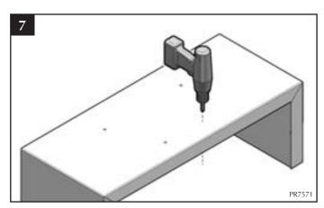
7. Drill four Ø8mm holes. Straight through both sides.
